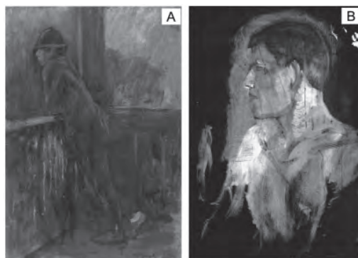
Fig. 1.: Comparison of the original (A) [3], and MA-XRF image of the Zn-L \alpha element (B) 180 degrees rotated. Both of the images were processed using graphic software.
